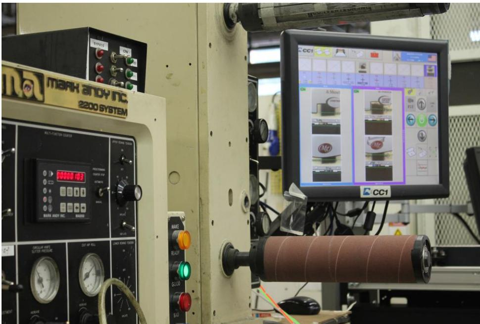
Recent retrofit installations of CC1's **DRC-6000L Camera-based Automatic Register Control** on Mark Andy presses are producing makeready savings of 50-75% in establishing color register.
