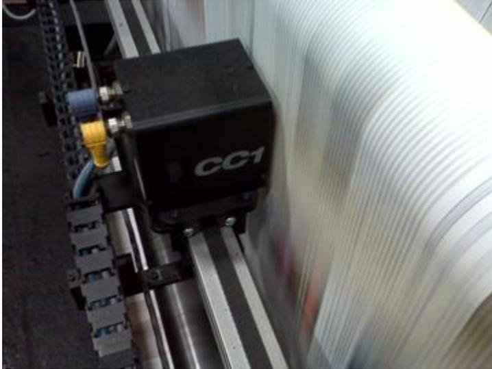
Featuring the latest in CC1's camera-based register control capabilities, the **DRC-6000L** automatically and precisely establishes register on startup, even if color marks overlap.
