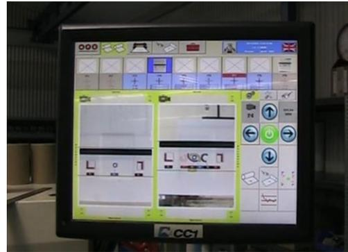
*CCI's DRC-6000L Automatic Register Control features smart camera technology and unique mark recognition algorithms for full automation of color register during make-ready. Final register can be established automatically even if color marks overlap.*
